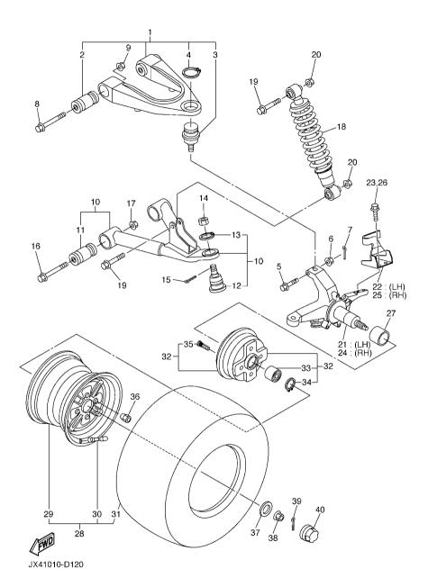
FIG. 3 FRONT SUSPENSION & WHEEL
